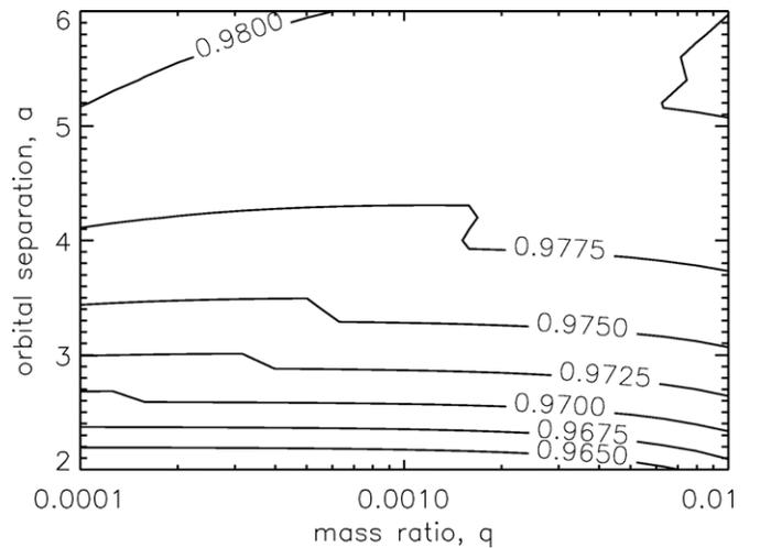
**Figure 4.** Ratio of the  $q$ -value estimated using the sinusoidal model (Equation (15)) and the actual  $q$ -value (shown along the  $x$ -axis) for a range of  $q$  and  $a$ . The sinusoidal model always underestimates the actual mass ratio by a few percent, and the estimate’s accuracy degrades for  $a \rightarrow 1$  as higher order Fourier components contribute more.
